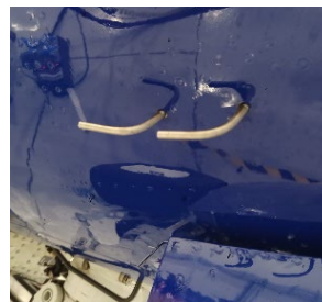
Figure 9 Sensor inlets from left to right: Rosemount, flushed mount, Chilled Mirror inlet, Flyht TAMDAR. Courtesy of FAAM Airborne Laboratory and FLYHT
